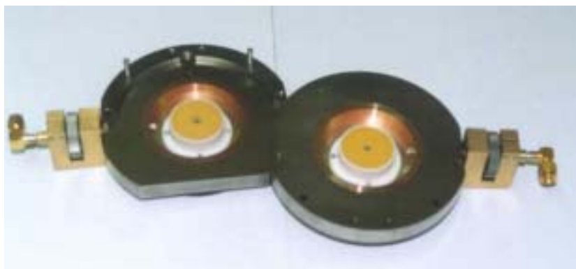
Fig.2 Photograph of disassembled 3.2 GHz split post dielectric resonator
