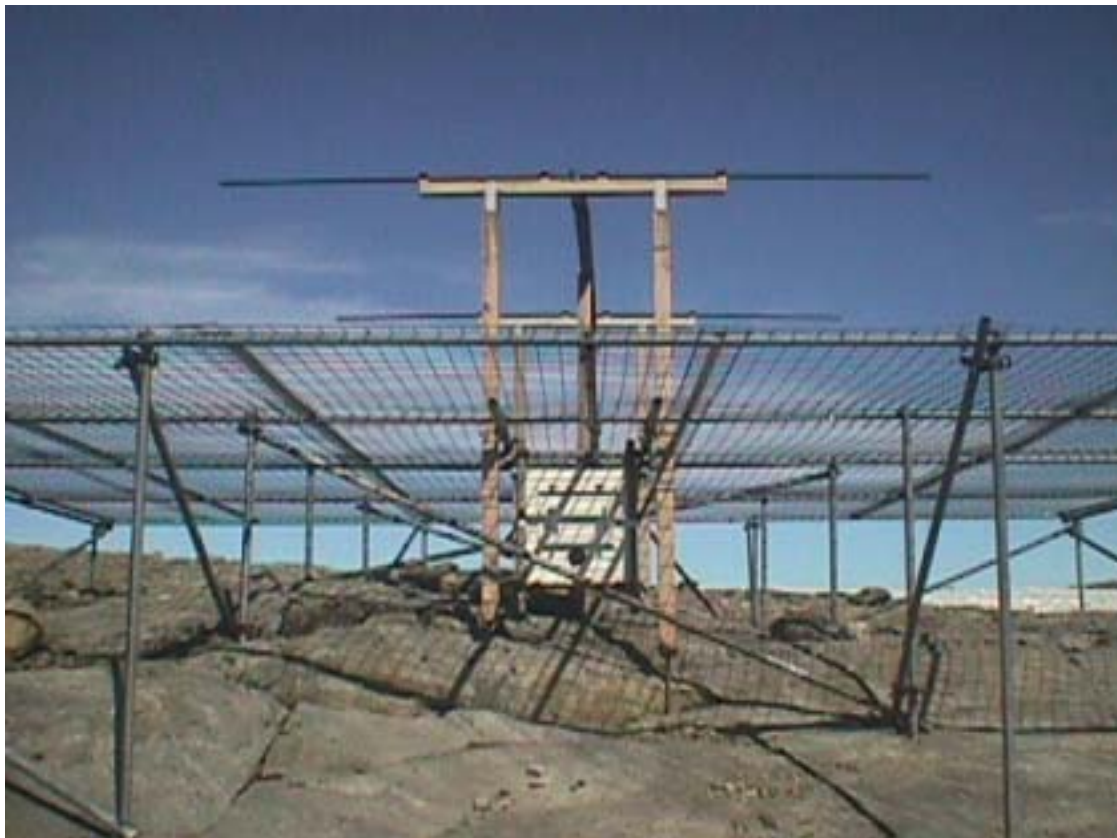
Fig. 2: A complete riometer system installed at Casey Antarctic station showing riometer, dipoles and the elevated ground plane
