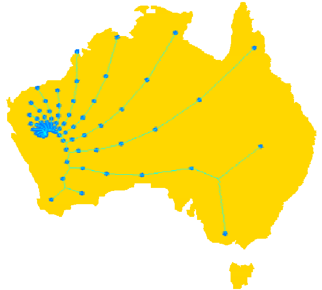
Fig. 1. A possible layout of the SKA across Australia showing 300 stations connected by optimised cabling [39]. For this realisation, each station would be in the order of 250m in diameter.
