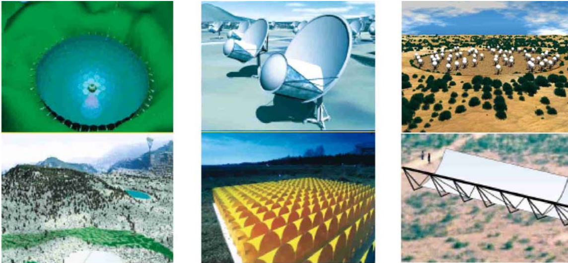
Fig. 1. SKA concepts. The left panel shows two large adaptive reflector ideas, one based on a 200 m diameter Arecibo-like spherical reflector (upper), the other using a much flatter reflector and an aerostat mounted focus cabin. The middle panel (upper) shows proposed 12 m diameter offset paraboloids, similar to the 6 m versions used in the Allen Telescope Array; the lower illustration shows a single-polarization Vivaldi-horn aperture phased array antenna under test. The right panel (upper) shows a station based on 64 x 7 m diameter Luneburg Lenses; the lower visualization is of a station employing a single 110 m x 15 m cylindrical reflector. The concepts originate in China, Canada, the USA, Europe and Australia (both right hand panels). Not shown is a 12 m symmetrical paraboloid proposed by the Indian SKA group.
