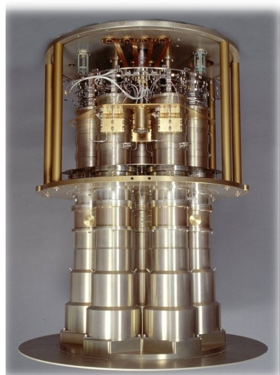
Fig. 4. Photograph of the assembled receiver with the cryostat wall removed to show the interior
