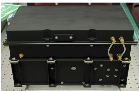
Communications Payload with Ka-band, UHF and On-board Processing Units
